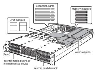
After installing internal options, check that the order and place of installation is correct and cables are correctly attached.
